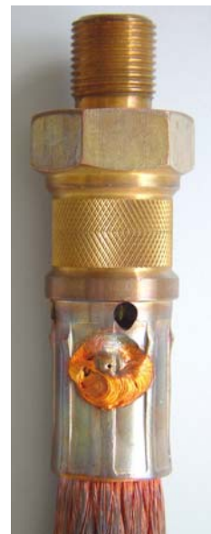
Copper wire and terminal welded together to improve the resistance
